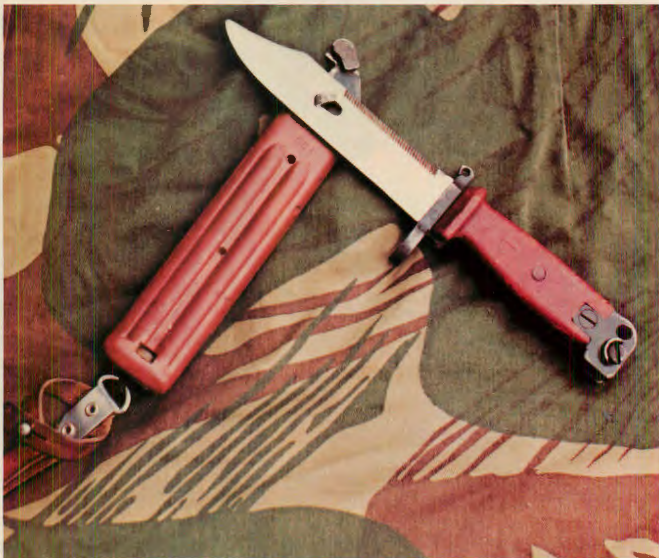
AKM bayonet attached to scabbard, ready to be used as wire-cutting tool.
